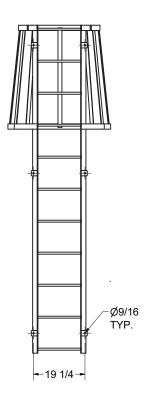
NOTE: STANDOFF BRACKET LOCATIONS ARE ± 1". DO NOT PREDRILL HOLES IN THE STRUCTURE. HOLES SHOULD BE MATCH DRILLED TO INSURE PROPER ALIGNMENT
