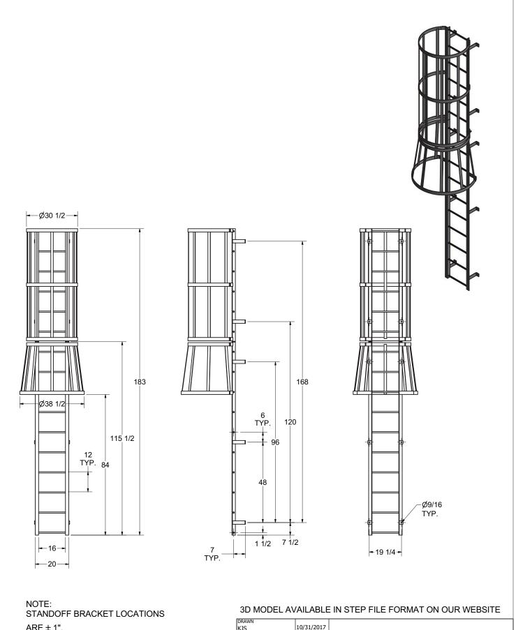
NOTE: STANDOFF BRACKET LOCATIONS ARE ± 1". DO NOT PREDRILL HOLES IN THE STRUCTURE. HOLES SHOULD BE MATCH DRILLED
