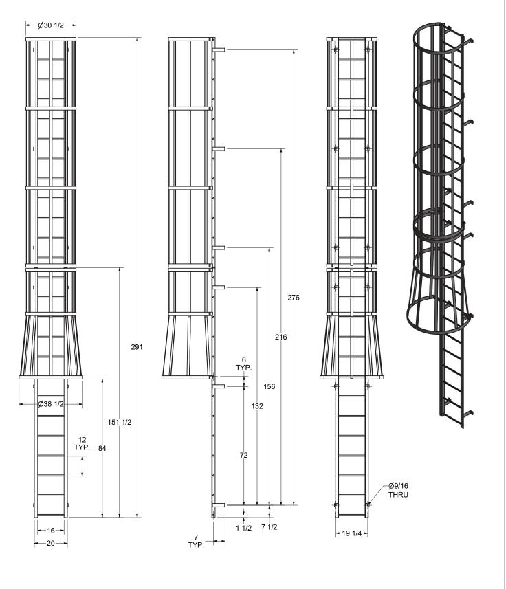
NOTE: STANDOFF BRACKET LOCATIONS ARE ± 1". DO NOT PREDRILL HOLES IN THE STRUCTURE. HOLES SHOULD BE MATCH DRILLED TO INSURE PROPER ALIGNMENT
